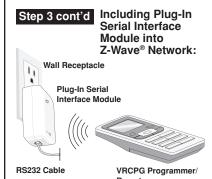
NOTE: Programmer/Remote must be in close proximity to Plug-In Serial Interface Module when including into network
