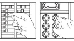
Next, plug in and turn ON the lamp or radio at the receptacle's other outlet to make sure the power is OFF at both outlets. If the power is not OFF, stop work and call an electrician to complete the installation.
