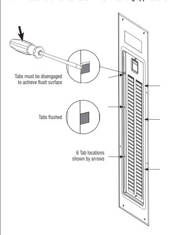
b. Adjustment screws in flush mounting applications.
