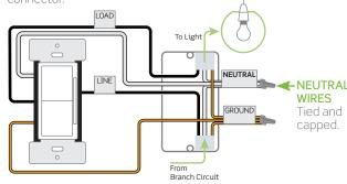
Quick tip: Check each individual location as some may have a Neutral wire and others may not. It is most common that a Neutral wire is missing in a wallbox where there is no bundle. Scan the code below for more information on how to identify a
