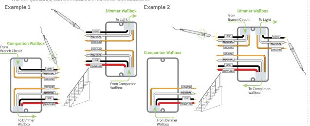
Most installations will match Example 1 or Example 2. If your wiring does not match either example, please contact Leviton Technical Support or consult an electrician.
