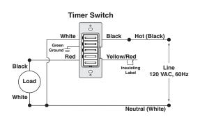
LTBxx Series 3-Way Wiring with Coordinating Remote Switch, VP0SR (no LED) Application
