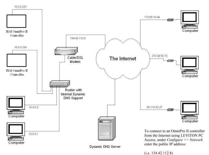
To connect to an OmniPro II controller on a local network using LEVITON PC Access, under *Configure* >> *Network* enter the controller's IP address:
